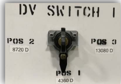
Figure 8 – Rotary multi-voltage switch
