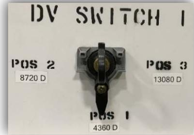
Figura 5 – Interruptor rotario multi-voltage
